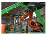
involving just one particular glass. In order to offer an esthetical seal between glass and body car, it is carried out on the glass periphery the Polyurethane extrusion, in particular on windshields, side fixed windows, backlights and roofs, by means of an application cell to be customized according to Client's requirements.
